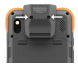
5. Route the hand strap through the hand strap mounting loop at the bottom of the barcode scanner expansion, if desired
