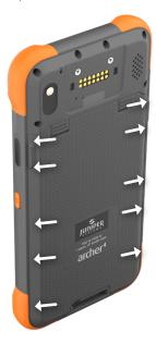
4. Slide the battery door locks into the locked position.
