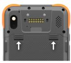
**A** CAUTION: The battery door latches must be in the locked position for the NFC to work.
